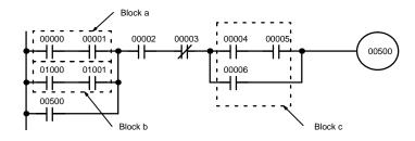
The first logic block instruction is used to combine the execution conditions resulting from blocks a and b, and the second one is to combine the execution condition of block c with the execution condition resulting from the normally closed condition assigned IR 00003. The rest of the diagram can be coded with OR, AND, and AND NOT instructions. The logical flow for this and the resulting code are shown below.
